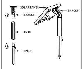
**6.** Insert the spike into the ground. Position the solar panel to face south (in northern hemisphere) to make the most of daylight hours. It is important to angle the solar panel towards the sun when sun is at its highest point. Ensure the solar panel is not shaded by trees, shrubs or buildings.
