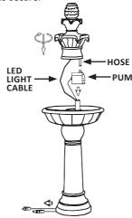
**4.** Fill the fountain with water, ensuring the pump is completely submersed.
