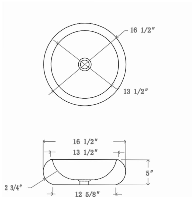
Dimensions of fixture are nominal and may vary within the range of tolerances established by ASME Standard A112.19.2. Dimensions and specifications subject to change without notice.
