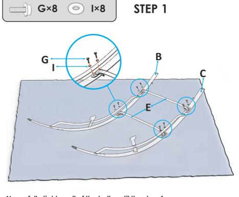
• Never fully tighten all of the bolts until the step 4.
