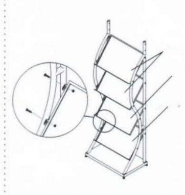
Fix the advertising board on the left and right brackets with screws and nuts;
