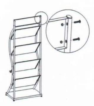
Adjust the magazine rack and tighten the screws to complete the installation.
