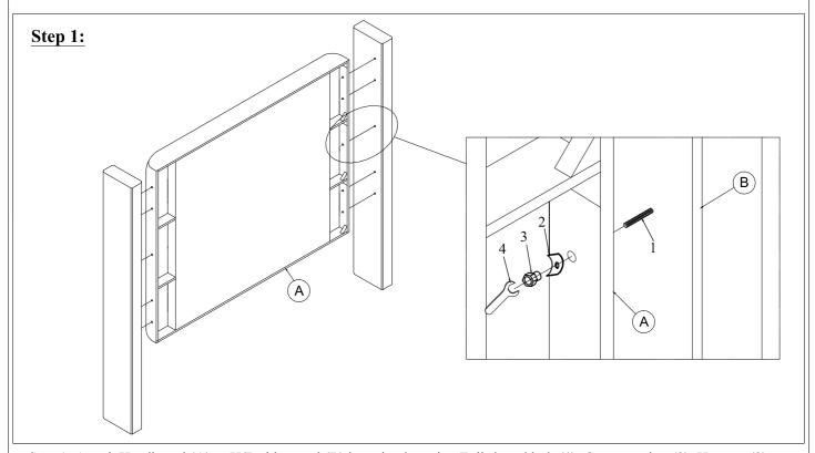
Step 1: Attach Headboard (A) to H/B side panel (B) by using by using Full-thread bolt (1), Curve washer (2), Hex nut (3) and Open wrench (4).
