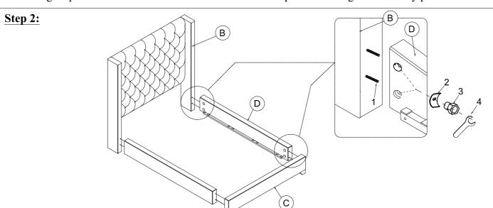
Step 2: Attach Bed side rail (D) to Footboard (C) and H/B side panel (B) by using Full-thread bolt (1), Curve washer (2), Hex nut (3) and Open wrench (4).
