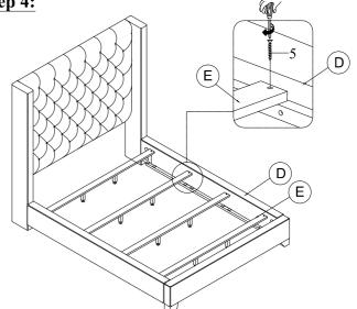
**Step 4:** Attach Slat (E) to Bed side rail (D) by using Screw (5) and Screw driver (not include).
