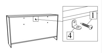
Locate the other bracket on the wall over a wall stud and two inches below the mounting bracket secured to the back of dresser. Attached to the wall stud using the long screw provided, through the smaller hole
