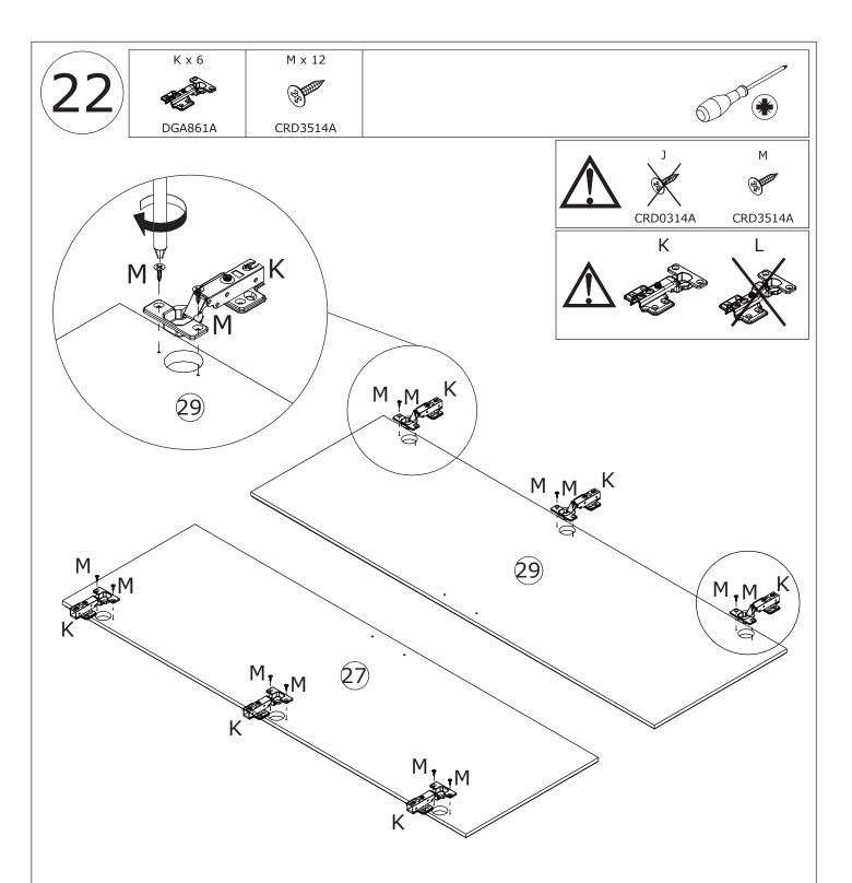
Fix hinge(K) to plate 27 and 29 respectively using screw(M) as shown. Please note, hinge(K) is used in this step.
