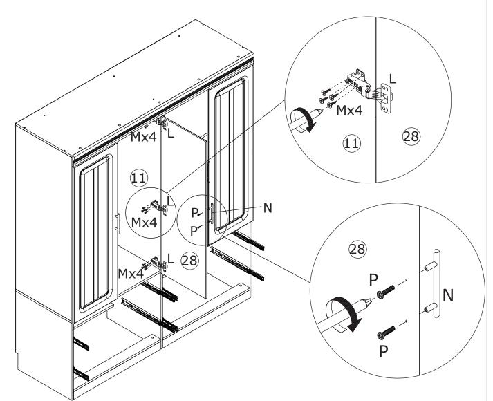
Attach plate 28 to plate 11 by fixing hinge(L) with screw(M) as shown. Fix handle(N) using screw(P) as shown.
