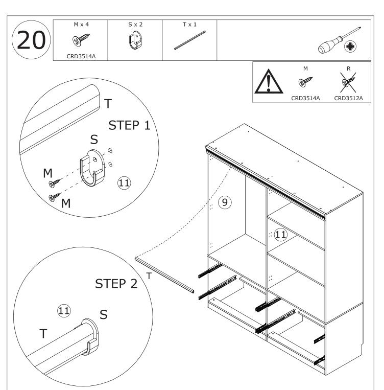
Fix part(S) to plate 9 and 11 using screw(M) as shown. Place clothing rod(T) as shown.
