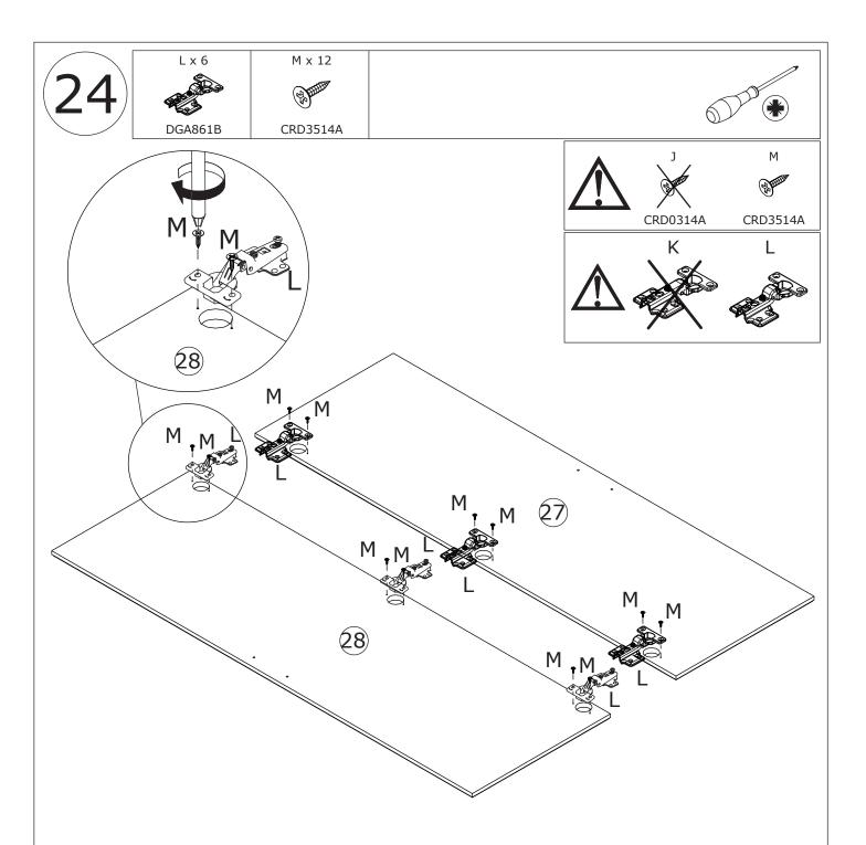
Fix hinge(L) to another plate 27 and 28 respectively using screw(M) as shown.
