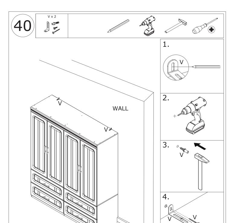
Install anti-tipping device(V) as shown.
