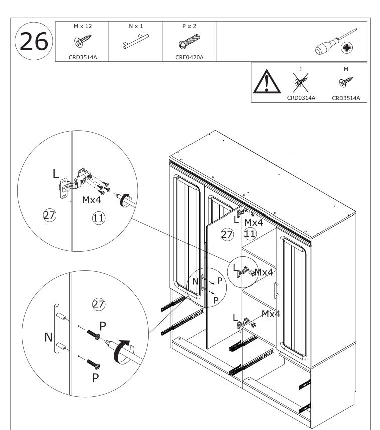
Attach plate 27 to plate 11 by fixing hinge(L) with screw(M) as shown. Fix handle(N) using screw(P) as shown.
