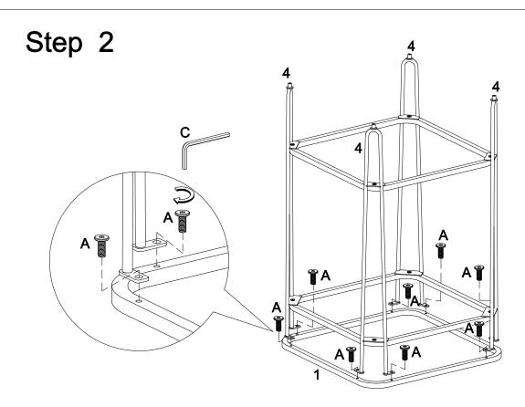
Use wrench (C) to secure top frame (1) to leg (4) with bolt (A).
