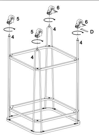
Screw caster (5,6) to leg (4), then tighten with wrench (D).
