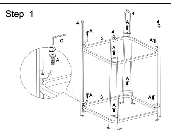
Use wrench (C) to secure shelf frame (3) to leg (4) with bolt (A).
