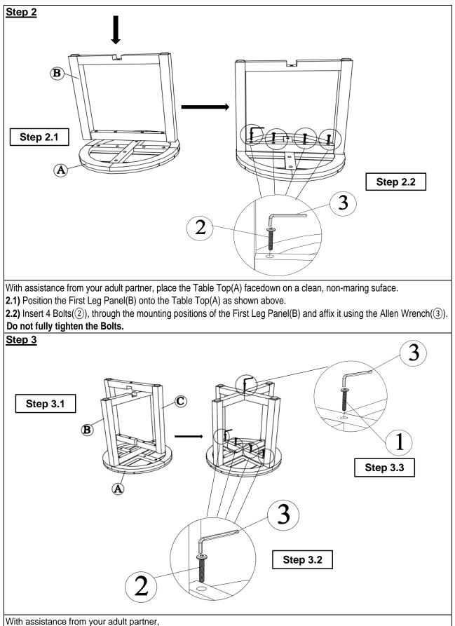
3.1) Position the groove point of the Second Leg Panel(C) over the First Leg Panel(B) in assembled part in Step 2.
