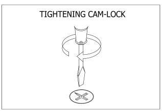
Use a Flat Screwdriver to turn Cam-lock clockwise so it locks onto the head of the Cam-bolt. Turn until it is snug (about one half a turn) -- over-tightening could damage Cam-lock or/and Cam-bolt.
