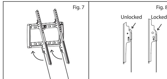
**IMPORTANT!** Verify that both arms are locked to the wall plate. For safety reasons, this mount cannot be used unless both arms are securely locked (see Fig. 8).
