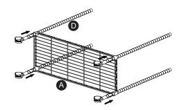
3. Turn assembly upright and push the shelf (A) firmly onto the tapered locks (B). Note: Make sure the lip of shelf (A) is facing down and the casters( E ) on bottom poles (D) are on the floor.
