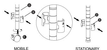
Attention: The tapered must be fixed to the groove on the pole, and make sure the tapered does not slip before installing the shelf
