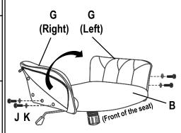
Using screws (J) and washers (K), assemble the backrest (A) to both armrests as shown. You can now tighten the screws and zip up the covers.
