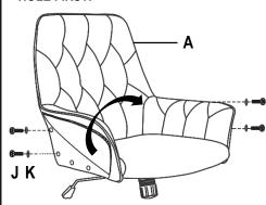
Place the top parts over the base parts making sure the tip of the gas lift enters into the hole of the mechanism.
