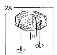
Carefully pull house wires through opening in center of mounting plate. With mounting plate threads facing outward, screw mounting plate into junction box using outlet box screws.
