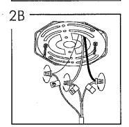
Strip 3/4" of insulation from wire ends. Connect house ground wire to fixture ground wire marked with symbol. Twist wires together using wire nut. Connect black house wire to the fixture wire marked "L". Twist wires together using wire nut. Connect white house wire to the fixture wire marked "N". Twist wires together using wire nut.
