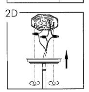
Lining up threads on mounting plate with holes in fixture canopy, attach fixture to junction box using cap nuts. Be sure to carefully tuck wires into canopy while attaching.
