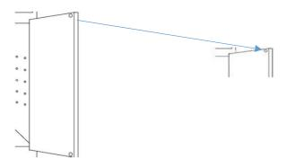
Using the wood glue, squeeze a small bead of glue in all grooves before assembling the cabinet sides, bottom, top and back panels. Be careful not to use too much glue, this could cause access glue to squeeze out and onto the panels, if this should happen, be sure to remove quickly.
