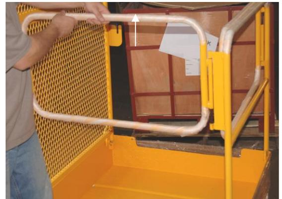
**Step 5: Secure the platform to the tines of the fork lift both tine locks and the (yellow) Nylon safety strap.**
