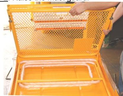
Lift the guard to allow the pegs to fit into the slots.
