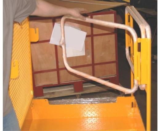
Lift the gate to allow the slots to slide onto the pegs welded to the toeboard.
