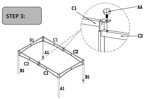
Now we have to assemble the 2 parts of Step 2 together.
