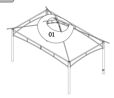
Now we are going to place the Big canopy (01) above the frame first. And make sure the frame of skylight is on top of the 01.
