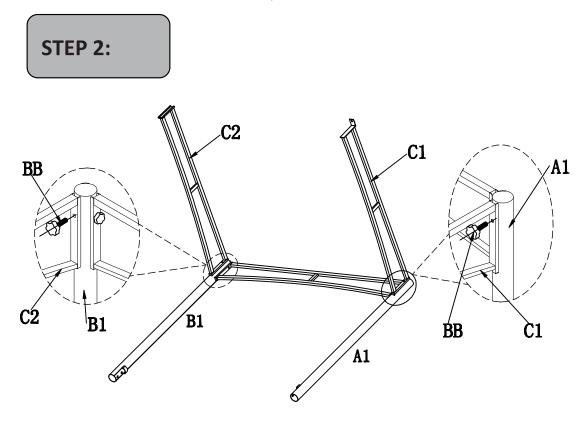
Based on Step 1, we have to assemble C1 into leg (A1) by using Screws (BB) And assemble C2 into leg (B1) by using screws (BB) too.
