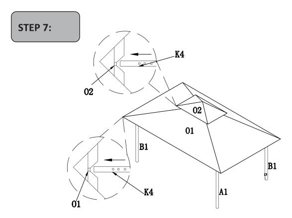
Please place the small canopy (02) above the skylight and Insert K4 into pocket and then adjust the tightness of the 02 in 4 sides
