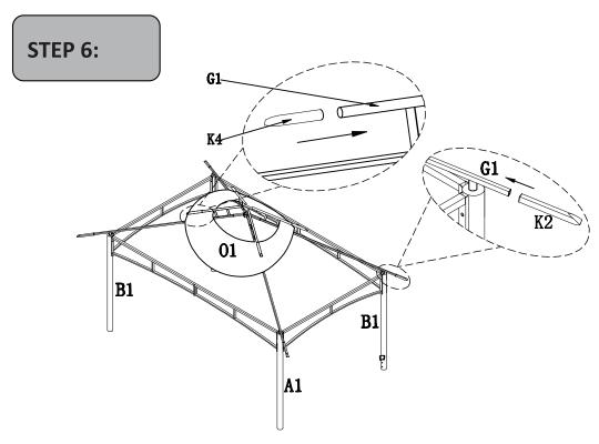
After Step 6, we need to assemble the Telescopic rods (K2) into the end of G1 as picture shows.
