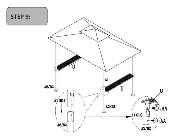
Please assemble the second Legs (A1/B2) into each leg, and do not lock them with screws first. We have to place the U part into the card slot on the legs at the same time then lock up by screws AA.
