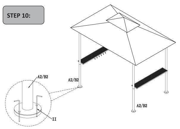
Finally, we have to insert the long screws II into the holes at the bottom of each second legs. To make sure this BBQ gazebo is strong enough.
