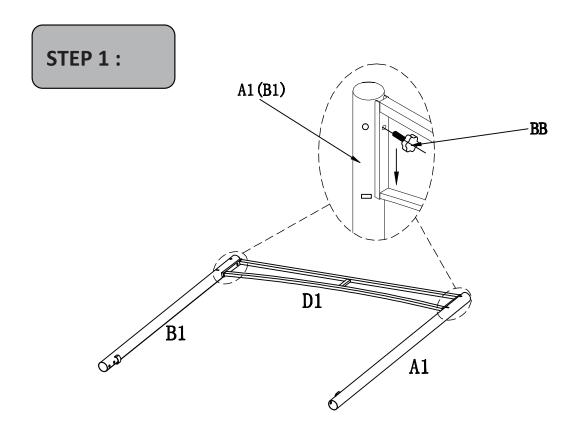
Please assemble legs of B1 and A1 into Side Beam (D1) by using screws (BB) We need to assemble 2 sets of above parts.
