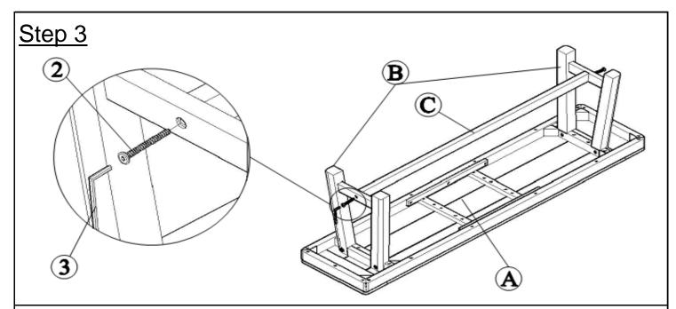
Insert the tenon of the Leg Support Bar(C) into the mortise of Leg Panels(B) . Attach Leg Support Bar(C) to Leg Panels(B) using Screws(2) with Allen Key(3) as shown above.
