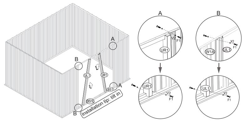
**Tips:** Insert UL1 and UR1 between the top beam and bottom frame respectively, and then push them to the corresponding position.
