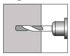
Using the drill bit size recommended on your wall anchor hardware, (not included) drill a hole equal to the depth of your anchor. \*Anchor hardware should be rated for the weight of your artwork or more.
