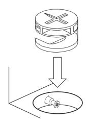
Turn the cam lock clockwise to tighten.
