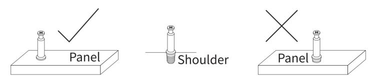
The pre-inserted nut should align with the center of the cam lock when joining two panels. The cam lock should be inserted before the eccentric wheel.
