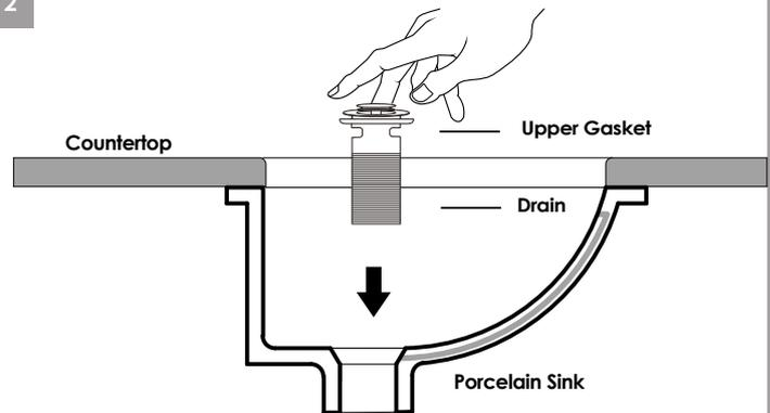
Introduce drain including upper gasket from the upper side of the sink.
