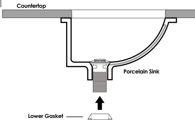
From underneath the countertop, insert lower gasket on the threaded area of the drain.
