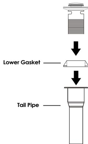
Remove lower gasket and tail pipe from the threaded shroud.
