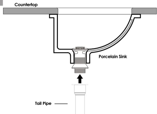
Secure the tail pipe, it is recommended to add Teflon to pipe threads, this tail pipe fits 1-1/4 inch home plumbing piping
