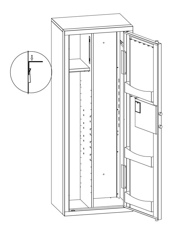
**Step 6:** Snap the internal cabinet base plate into the slot.
