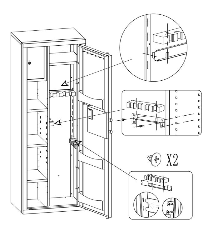
**Step 9:** Install the 3 types of gun racks as shown in the picture.
