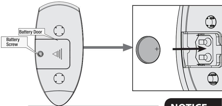
To access the battery compartment, remove the small Phillips head screw that secures the battery door to the transmitter assembly. Install one 3-Volt, CR2032 battery, found in the remote control hardware bag, into the transmitter. Clean the battery contacts and also those of the device prior to battery installation. The battery should be installed with the positive (+) side up. Please contact your local battery recycling center for proper battery disposal information.
