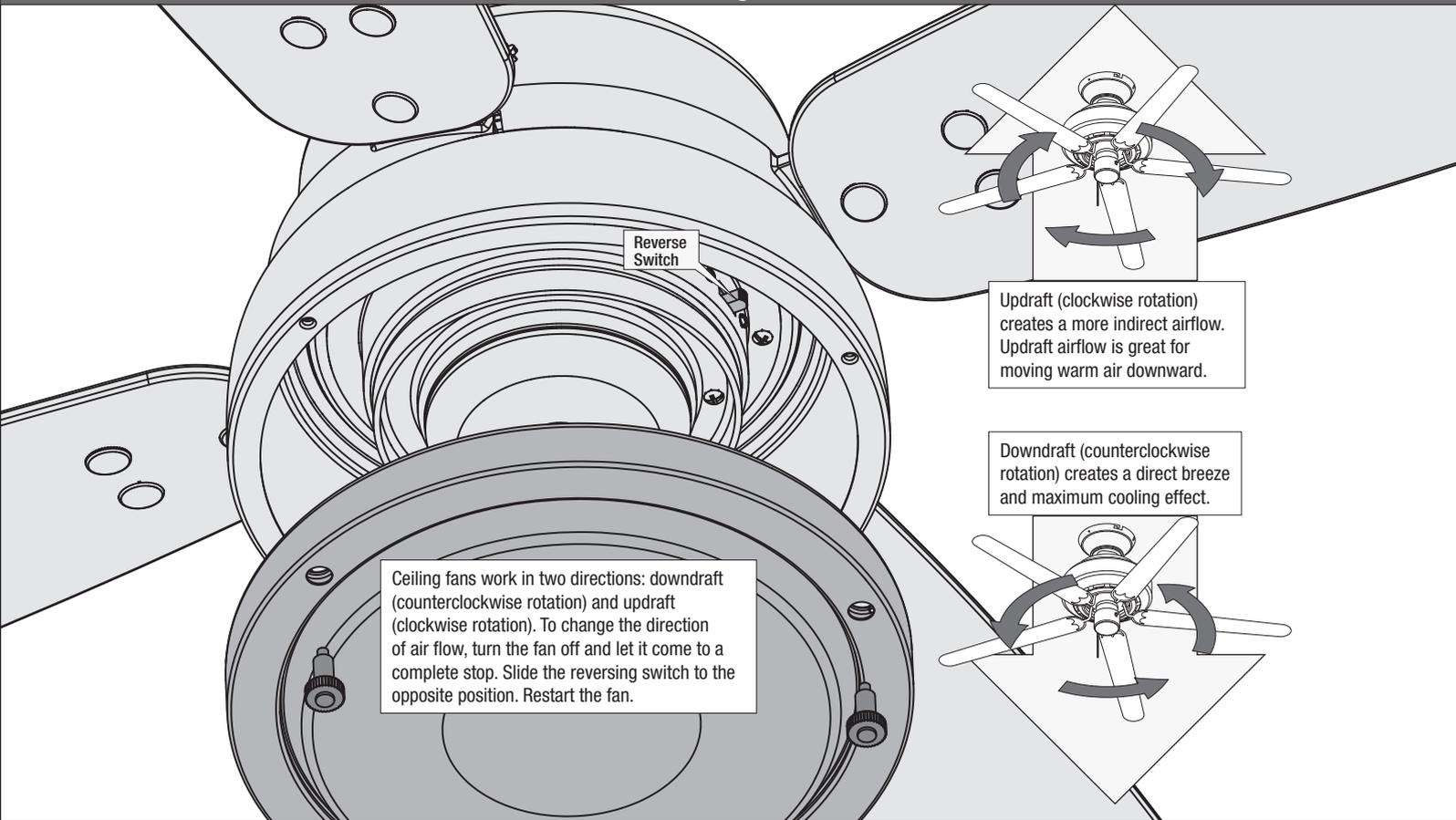
Ceiling fans work in two directions: downdraft (counterclockwise rotation) and updraft (clockwise rotation). To change the direction of air flow, turn the fan off and let it come to a complete stop. Slide the reversing switch to the opposite position. Restart the fan.
