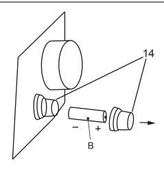
6. Remove the Electronic Ignitor Cap (14) on the electronic Ignitor (14) by unscrewing and slide the Battery (B) into the battery slot (14).
