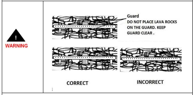
To ensure proper function, the Guard (01) on the Burner (08) should never have lava rocks (A) covered over it.
