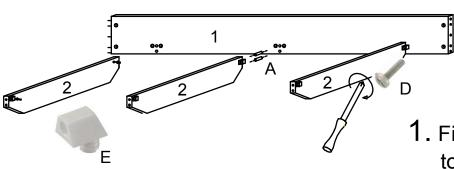
1. Fit the slat supports to the side rail, using the screws 4MA
