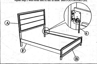
STEP 3: Tighten the 4 Corner with Allen Key (6). Fix the Bed Slat Support Leg (E) to Bed Slat (D). Install the bed slat (D) to side rail (F) and tighten with Csk Screw (1) as per diagram shown. (NOTE: THE SETUP MUST DONE AT THE DECIDED LOCATION FOR THE BED TO OBTAIN PERFECT STABILITY)
