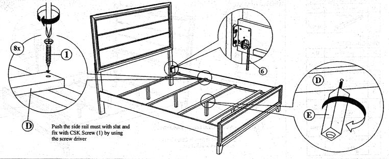
NOTE: MUST TIGHTEN SCREWS PERIODCALLY WITH USE SCREW WILL BECOME LOOSE CHECK TIGHTNESS OF ALL SCREW EVERY 6-8 WEEKS.
