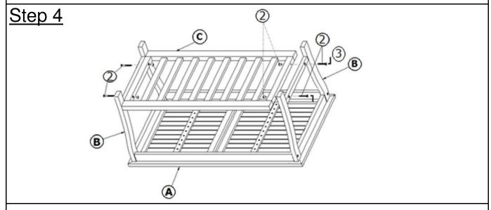
Affix Shelf (C) to Leg Panel (B) by using Bolts & Sleeve Nuts (2) and Allen Key (3). You may need to push the Leg Panels (B), outwards, slightly to attach the legs. **LOOSELY TIGHTEN THE SCREWS, up to 80%.**
