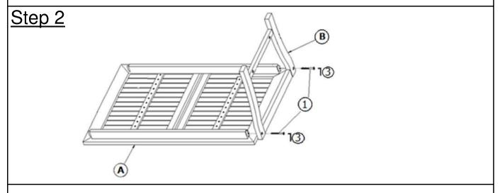
Position Table Top (A) and Leg Panel (B) as shown in picture above. Then affix 1st Leg Panel (B) to Table Top (A) by using Screws (1) and Allen Key (3) LOOSELY TIGHTEN THE SCREWS, up tp 80%.
