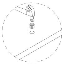
Note, please use a tool to carefully align the plastic pellets with the holes and then knock them down
