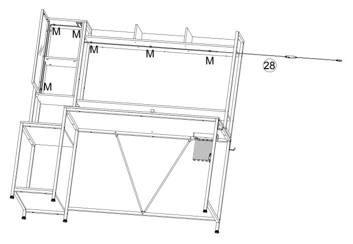
Note that M can be installed or not according to personal needs. M is used for the stick-off configuration of the light strip.
