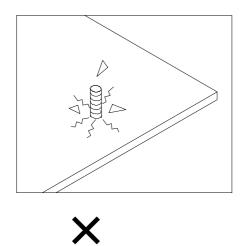
Wrong screws can cause the plank to crack
