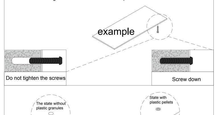
Note that if you find that there are no plastic granules on the wooden block, the table cannot be assembled, please don't worry, please use the spare plastic granules in the screw bag
