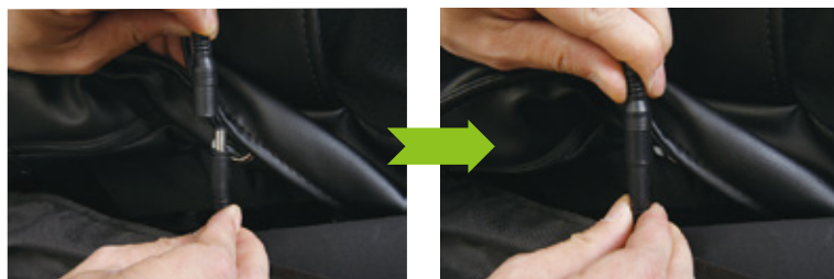
Connect back cushion heat wire.
