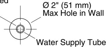
For slip-fit spout, 5/8" OD tube must extend 2-1/2" (64 mm) beyond finished wall.
