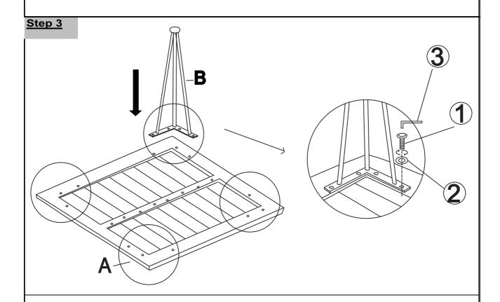
Attach Leg(B) to Table Top(A) using Bolts(1), and Washers(2), with Allen Key(3). **Do not fully tighten the Bolts.**
