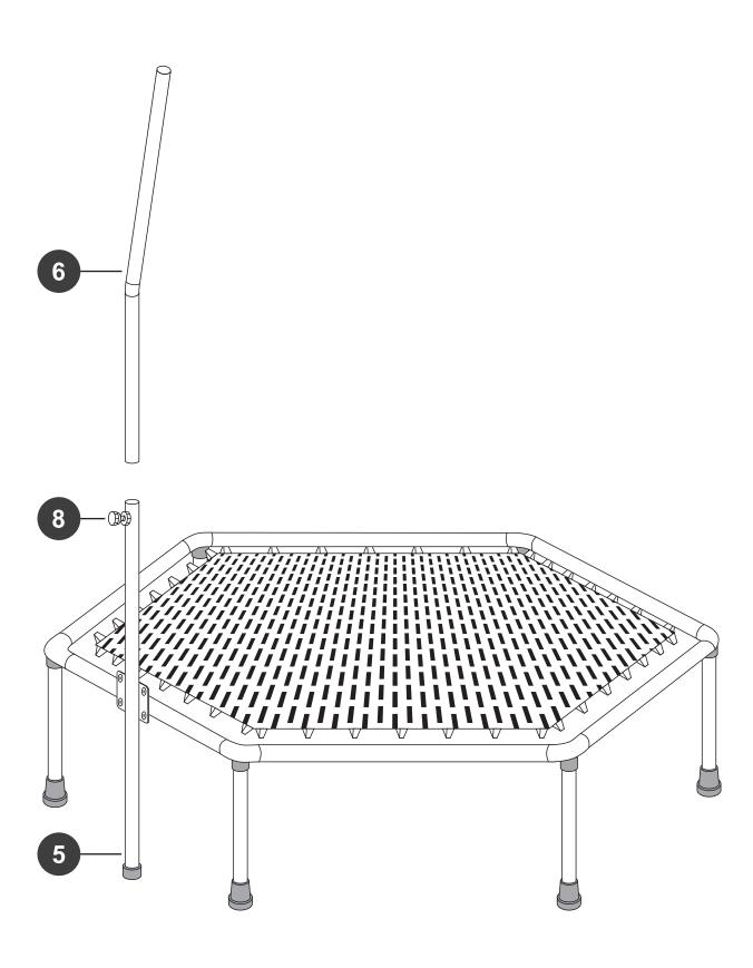
**Step 7 -** Assemble the handrail (Manual item #7) to the upper handrail support (Manual Item #6). Attach the handle by using the screws (Manual items 12 and 14), and tightening the screw with the wrench, as shown in the picture below.
