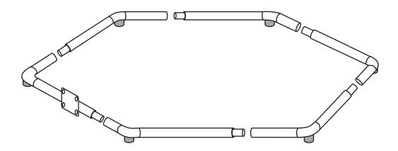
**Step 2 -** Remove the black caps that cover the leg connectors. Screw all legs onto the frame leg connectors. (It is the small threaded pieces that extends from the frame.)
