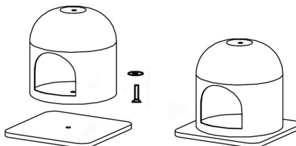
2. Attach the Sisal-Wrapped Tube (F) to the Dome Cubby (D). Turn clockwise to tighten.
