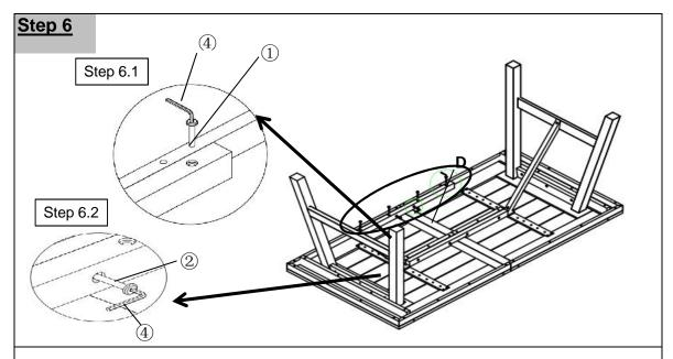
Position Side Support Bar(D) as shown in picture above.
