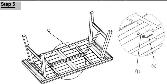
Position Middle Support Bar(C) as shown in picture above. Insert the four Long Bolts(①) through the mounting positions and affix the Middle Support Bar(C) to Table(A) using the Allen Key(④) Only loosely tighten the Bolts.
