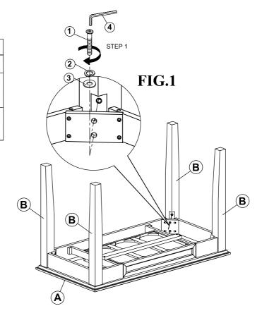
STEP 1: Place the Table Top(A) on the floor with a piece of cloth or carpet. Attach the Leg (B) to the top using provided hardware as shown on FIG.1.
