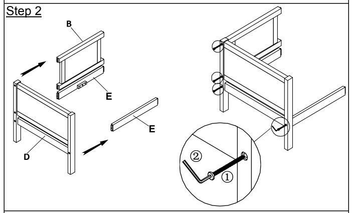
With the help of your adult partner, insert tenons of Backrest Panel (B) and Support Bar (E) into the mortises of the Left Panel (D) using Screw (1) with Allen Key(2) as shown in picture above.
