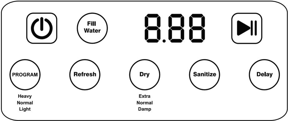
**On/Off Power icon** (power icon) - Powers on the Steam Dryer Closet. All the selections on the Control Panel illuminate.
