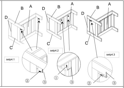
Step4.1:Attach Seat(A) and Backrest (D)to Left Side Panel(B) using Bolts(②) with Allen Key(③) as shown above.
