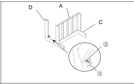
Attach Backrest(D) to Right Side Panel(C) using Bolts(②) with Allen Key(③) as shown above. Do not fully tighten the Bolts.
