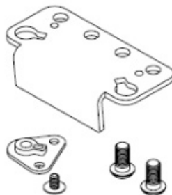
Figure 7a - Lower Hinge Bracket (Before Reversal)
