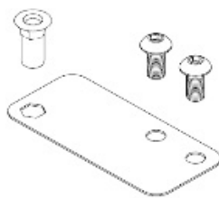
Figure 7 - Upper Hinge Bracket (Before Reversal)
