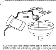
1. Carefully push the canopy to the bottom of the mounting bracket, make two sliding holes aligned to the two promine screws on the mounting bracket, and then turn clockwise until tight.
