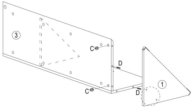
Note: The holes facing up during installation.
