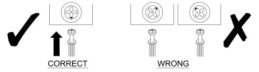
When fitting a cam lock, ensure the starting position is correct before inserting the connecting QUI CKFIT
