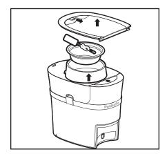
We recommend you wash and rinse the bowl, bowl holder, food hopper, lid and conveyor. Once parts are dry, ensure a conveyor belt lip is aligned with the arrows on the side. Replace the conveyor and food hopper.
