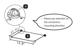
Before next step, please make sure to assemble the shelf corner to the end of the connector hole.
