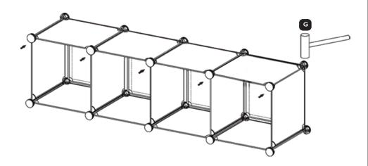
To tighten the connections between the parts, please knock down the connectors with a rubber hammer to ensure that the shelf corners are assembled to the end of the connector holes.
