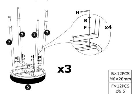
**Step 8:** Please do not tighten all bolts until the products is assembled completely.
