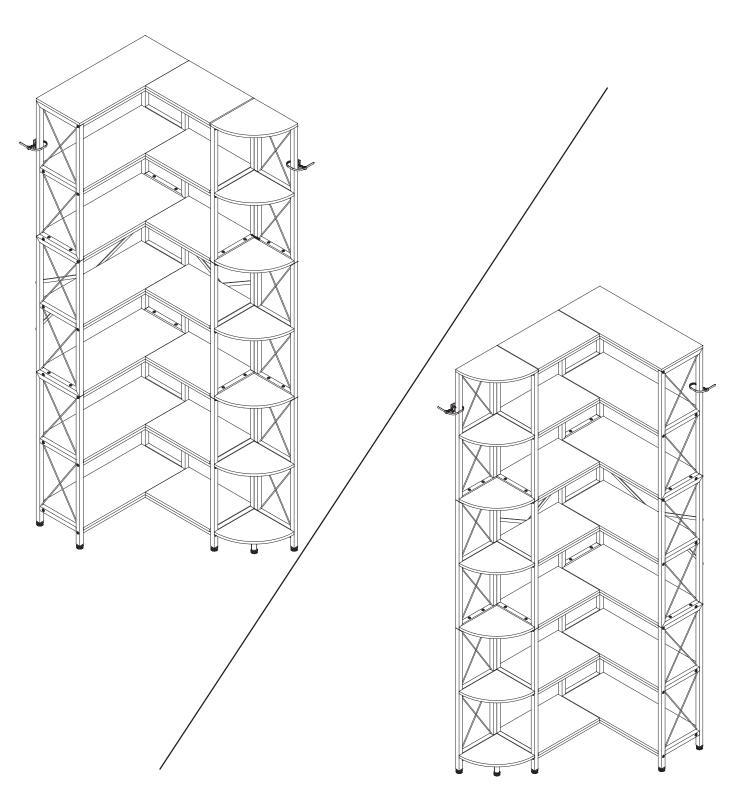
**Notes:** Don't tighten screws completely at first, just in case parts were assembled wrong and need be disassembled. Tighten screws at last when all parts are put together.
