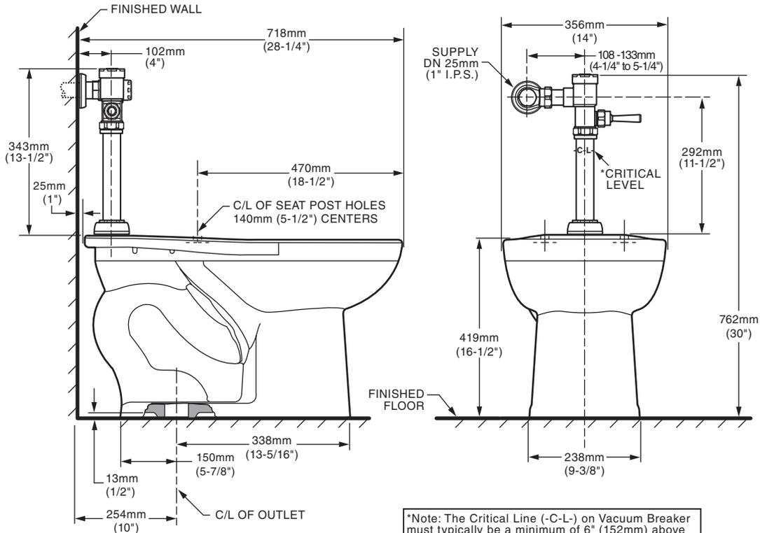
\*Note: The Critical Line (-C-L-) on Vacuum Breaker must typically be a minimum of 6" (152mm) above fixture. Consult Codes for details.
