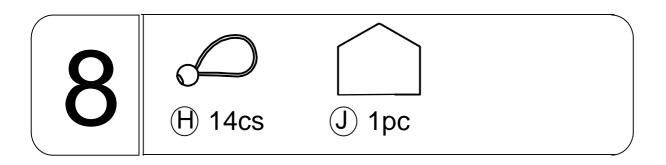
Fix the Back tarp (J) and Top tarp (D), Back tarp (J) and Tarp wall ( $\kappa$ ) by Elastic band (H).
