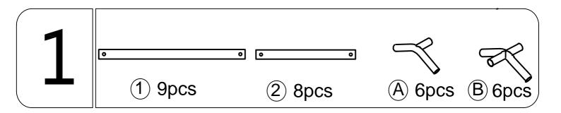
Put Long top tube (1), Short top tube (2), Three-way tube joint (A) and Four-way tube joint (B) in the shown order.
