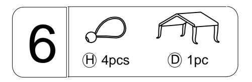
Put the Top tarp (D) on and fix it to the supporting tube by Elastic band (H).
