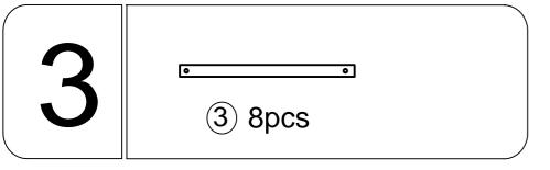
Insert the Supporting tube (3) into the tube joint (A) and (B) to make the structure as shown.
