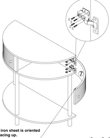
Note: The lock iron sheet is oriented with one side facing up.
