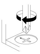
Turn cam lock clockwise to tighten.
